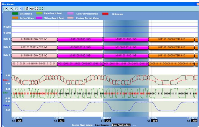
Figure 5: MHL Bus viewer with Physical layer waveforms
