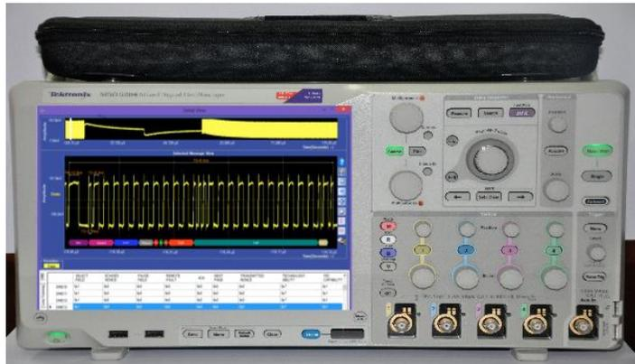
PGY-NEGO Software running on Tektronix oscilloscope
