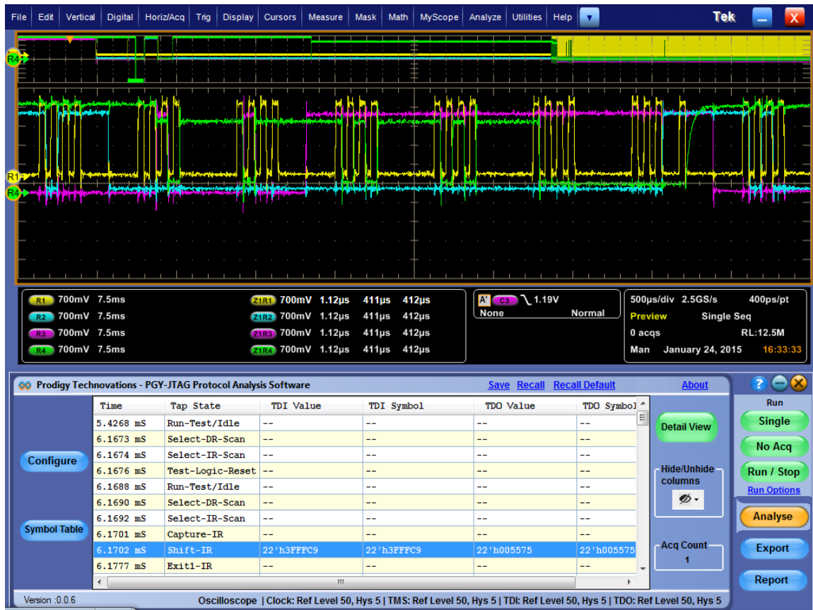
JTAG Protocol Analysis view in oscilloscope waveform display
