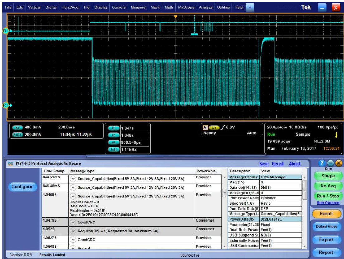
PD Protocol Analysis view in oscilloscope waveform display
