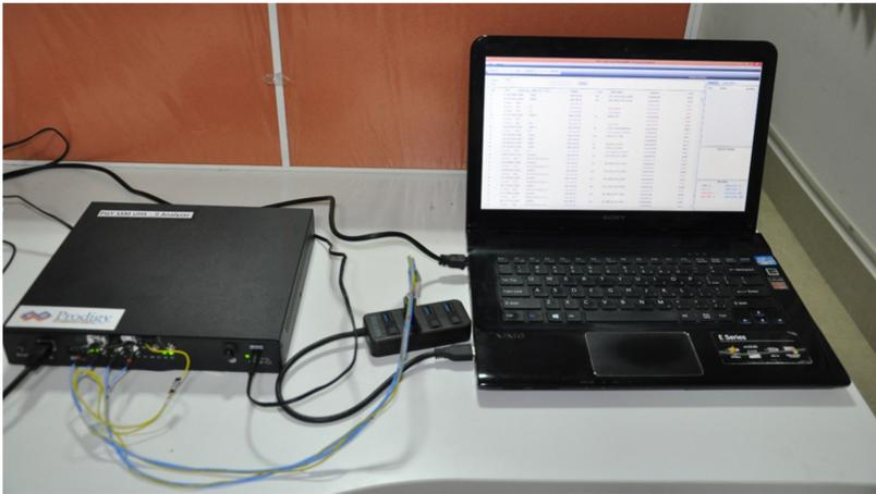
PGY-UHS II Protocol Analyzer provides USB3.0 and GBe interface for host connectivity. PGY-UHS II software runs in host machine enables configuration of PGY-UHS II hardware for UHS II protocol analysis storage
