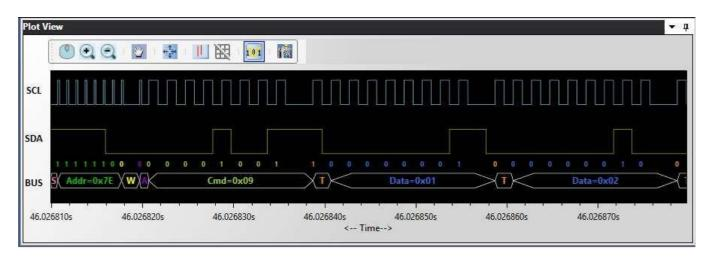
The timing view provides the plot of SCL and SDA signals with bus diagram information. Overlaying of protocol bits on the digital timing waveform helps in the easy debugging of protocol decoded data. Cursor and Zoom features make it convenient to analyze protocol in timing diagrams for any timing error
