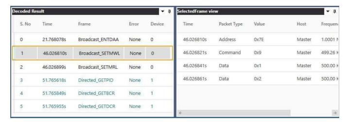
The protocol window provides the decoded packet information in each state and all packet details with error info in the packet. The selected frame in the protocol listing window will be auto-correlated in the timing view to view the timing information of the packet.
