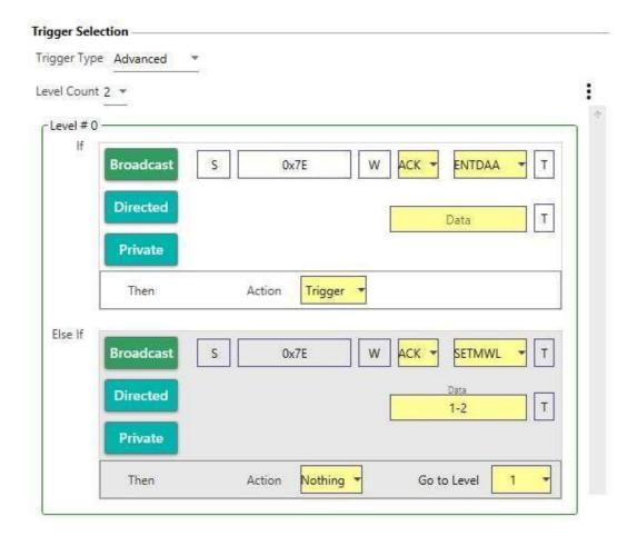
PGY-I3C-EX-PD supports auto, simple, and advanced trigger capabilities. The analyzer can trigger on any of the protocol packets such as broadcast, directed, or private messages. Advanced trigger provides the flexibility to monitor multiple trigger conditions and can set multiple state trigger machines.
