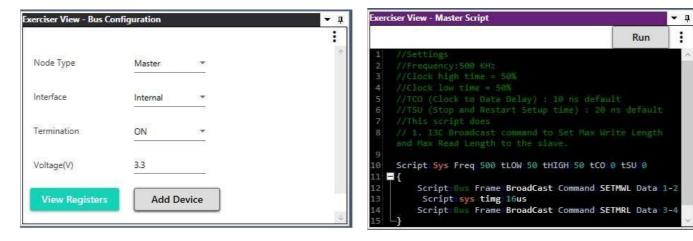
PGY-I3C-EX-PD supports I3C traffic generation using GUI and Script. Users can perform simple traffic generation using the GUI to test the DUT. Script-based GUI provides flexibility to emulate the complete expected traffic in the real-world including error injections. In the below sample script users can generate I3C traffic as below:
