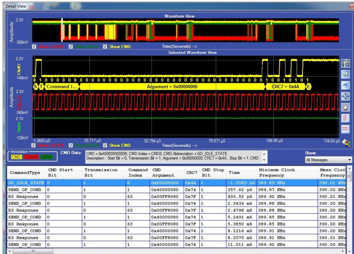
Detail View correlates Waveform, Protocol and electrical measurements
